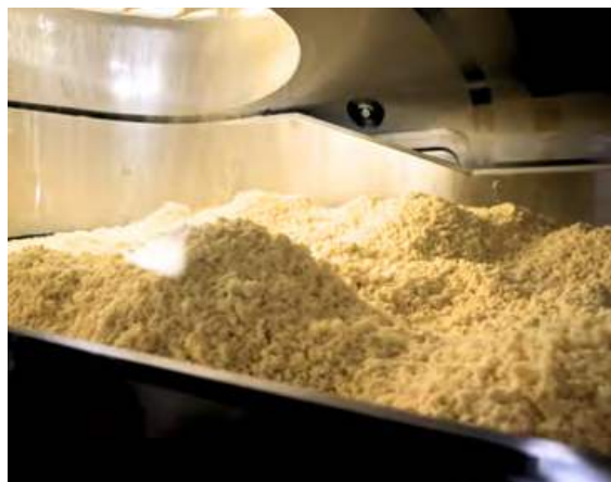
Figure 7: Image of powder falling from the spray dryer chamber onto the timing belt.
