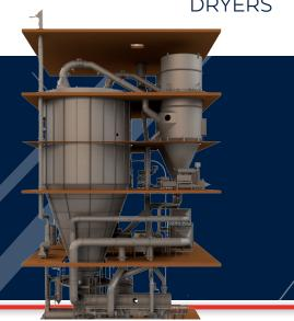
The L-TECH™ Permeate Drying System's Air Lift Dryer is fed from the bottom, increasing residence time. An integrated circular fluid bed at the bottom of the chamber provides second-stage drying and fines agglomeration. The recovered fines are conveyed to the drying chamber for agglomeration
