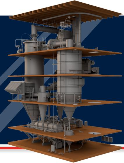
The Tall Form Bustle Dryer is optimized with a vertical hot air distributor, vibrating well mixed and plug flow beds and baghouse. Other features can be added for specific customer requirements and include: multi fuel indirect fired heater, timing belt, cyclones, baghouse fines retention bin, heat recovery, dual feed system, retractable cip nozzles, lecithination and spray nozzle cameras.
